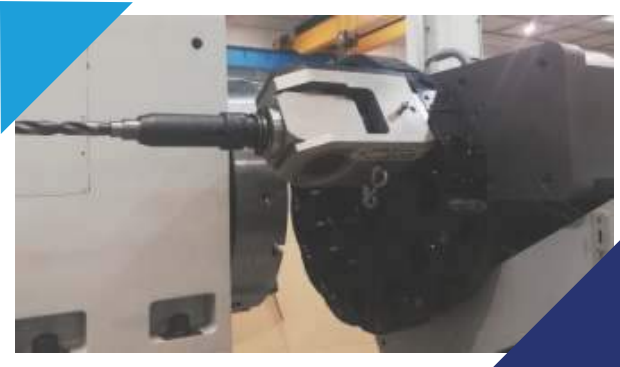
Moduli assiali e radiali per torretta a disco. Axial and radial live tool modules for disk turrets.
