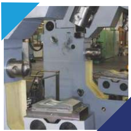
Lunetta a rulli con pattino idrostatico intercambiabile. Steady rest with rollers with interchangeable.
